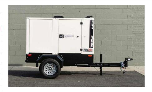
TecnoGen's 20kVA generator uses the Kohler engine coupled to an industry standard Leroy Somer alternator producing 17kW of prime power. Standard features include camlocks, and block heater. The Deep Sea controller makes retrieving vital stats like fuel levels, run time and start logs easy and the sealed doors and 2" thick insulation throughout gives this gen a 68dBA rating.
